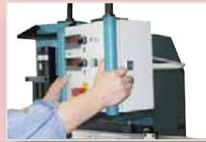
Control panel with two-hand operation
