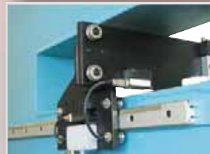
Distance measurement of X and Y-traverse paths
